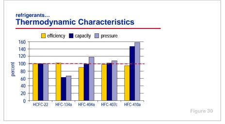
Today the most commonly used refrigerant in helical-rotary chillers is HCFC-22. Due to the scheduled phaseout of HCFC-22, most helical-rotary chillers will be redesigned using HFC refrigerants. Many challenges are encountered when redesigning a chiller to use a refrigerant with different thermodynamic characteristics. This is due to the different efficiency, capacity, and operating pressure characteristics of each of the refrigerants.
